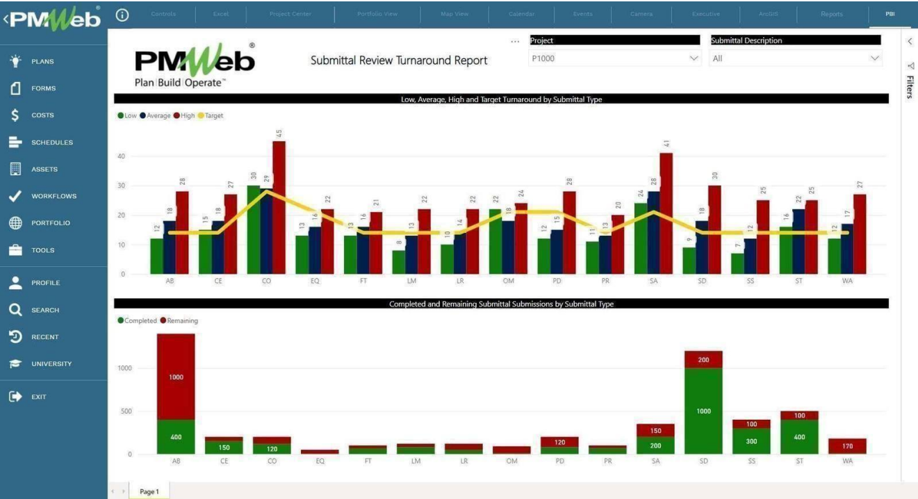
Submittal review turnaround report on PMWEB data: actual against target review durations, and completed and remaining submittals by type. Earlier PMWEB release; sample data.
