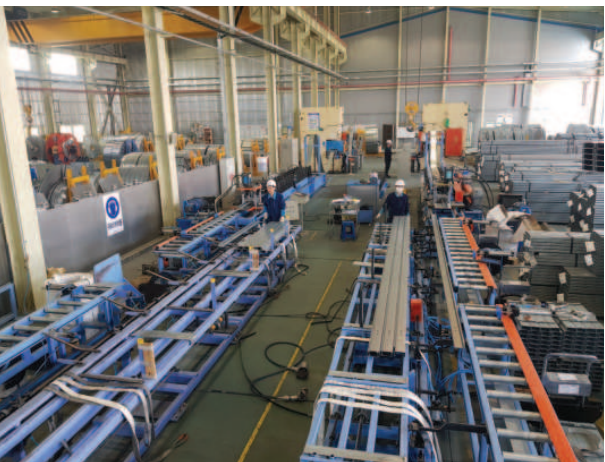
C-Channel Roll Forming Line Equipment that produces C-channels by performing hole punching at designated sizes and positions using a hydraulic press before the roll-forming process.
