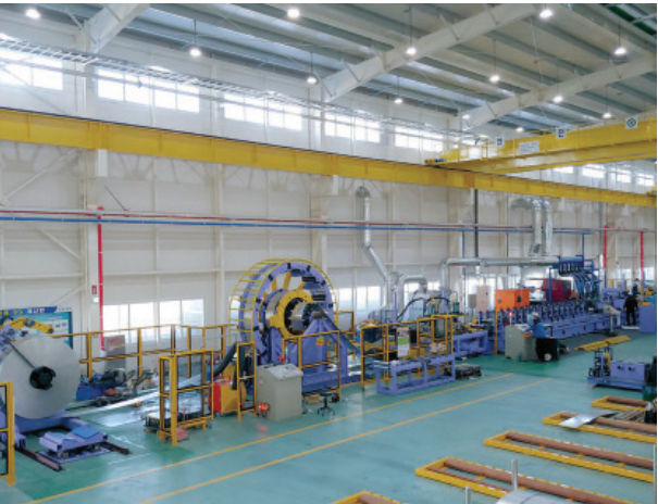
Pre-Punched Tube Mill Equipment that performs precision hole punching at designated positions using a flying punching system before the roll-forming process, ensuring both high production efficiency and machining accuracy.
