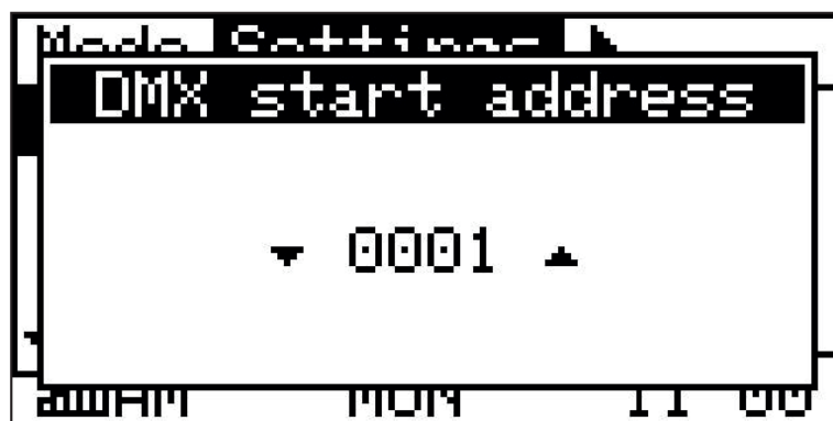
Figure 35: Setting the DMX Start address
