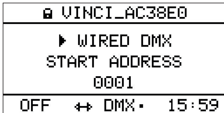
Figure 32: Controller configured in Wired DMX mode
