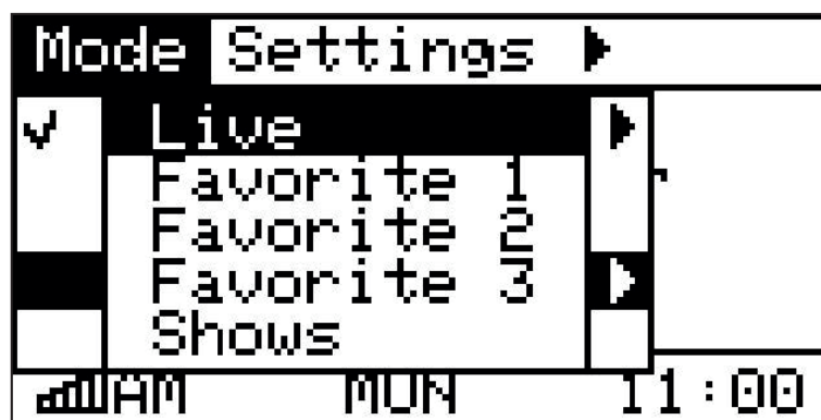
Figure 37: Setting a Sync Master to distribute a Live effect
