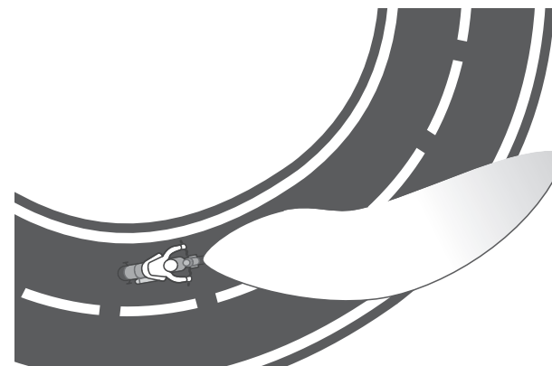
Adaptive high beam on (when cornering)
