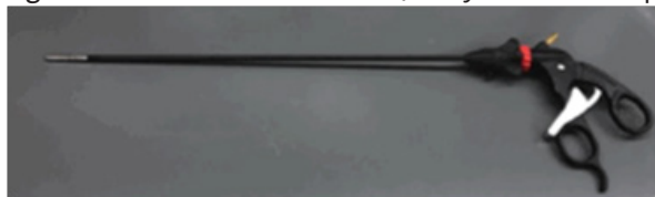
Figure 2: Custom-manufactured, wavy atraumatic laparoscopic graspers with non-ferromagnetic 316 stainless steel tips
