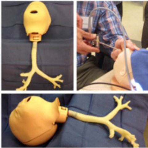
Figure 1: Assembled Retrieval of Airway Foreign Body Rigid Bronchoscopy Simulation Model Using 3D Printed 18-month old Tracheobronchial Airway
