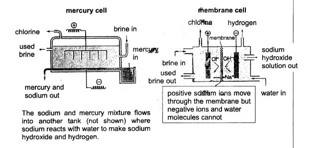
The membrane cell allows sodium hydroxide and chlorine to be produced in the same cell. Without the membrane, the sodium hydroxide would not be pure because it would contain chloride ions.
