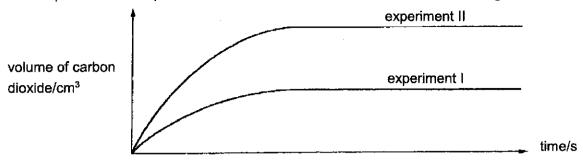
Experiment I was a reaction between excess calcium carbonate and 25 cm³ of 0.75 mol/dm³ hydrochloric acid. The volume of carbon dioxide collected in experiment II was twice the volume collected in experiment I.
