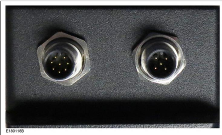
The ThermaWatch Rotor signal conditioner features two sockets. Note that connectors and sockets are keyed.
