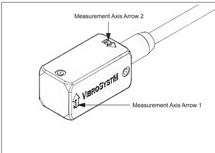
The FOA-200 is a dual-axis accelerometer. The arrows on the sensor head indicate the measurement axes and vibration directions corresponding to ascending electric signals.
