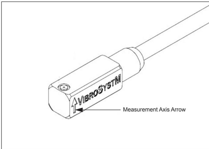
The FOA-100E is a single-axis accelerometer. The arrow on the sensor head indicates the measurement axis and vibration direction corresponding to an ascending signal.
