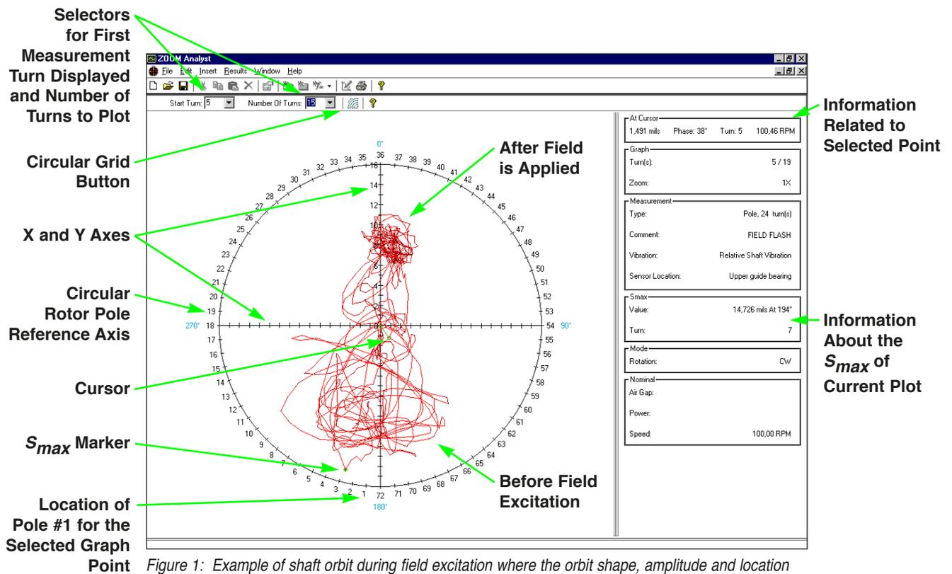
The orbit is traced by calculating the resultant vector ( $S$ )<sup>2</sup> summation from the X and Y proximity probes located at the guide bearings. As ZOOM synchronizes data acquisition of vibration inputs to the passage of each rotor pole during a machine turn, it provides a number of samples per rotation equal to the number of rotor poles. Therefore, the resultant vector is relative to rotor poles instead of degrees.
