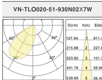
Above test data is based on 3000K 90CRI LED
