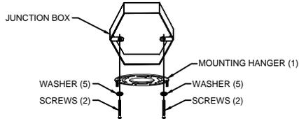
Secure the mounting hanger (1) to the electric junction box with the screws (2) and washers (5) provided.
