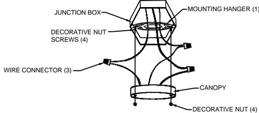
Install the canopy (shade/cover) of the decorative fixture to the mounting hanger, using the supplied screws or decorative nuts (4).
