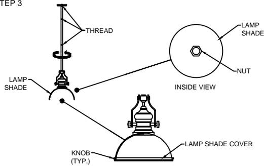
Thread the extension arm together, securing by hand pressure. Install the lamp shade by threading the nut clockwise from the inside. Install the recommended bulb into the socket and install the lamp shade cover by threading the three knobs around the sides by hand pressure.
