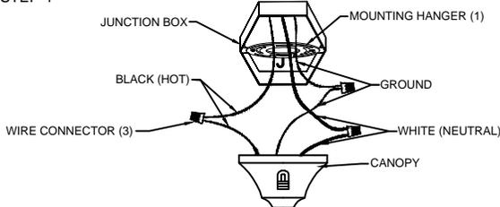
Connect the hot wire from main wire to the hot wire from power supply. Connect the neutral wire from the main wire to the neutral wire from power supply. Fix the ground wire from fitting to ground wire (grounding) from power supply.
