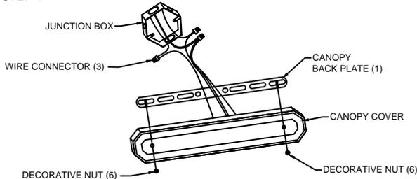
Install the recommended bulbs in the sockets and then install the canopy (shade/cover) of the decorative fixture to the mounting hanger, using the supplied screws or decorative nuts (6).
