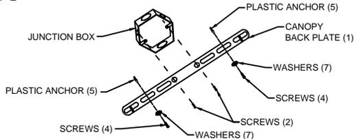
Secure the canopy back plate (1) to the electric junction box and the ceiling with the screws (2 and 4), washers (7) and plastic anchors (5) provided.
