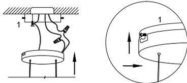
Mount the fixture ceiling canopy to the hanger by sliding the fixture cover over the hanger where the screws are sticking out on the side and twist to the right to lock into place.
