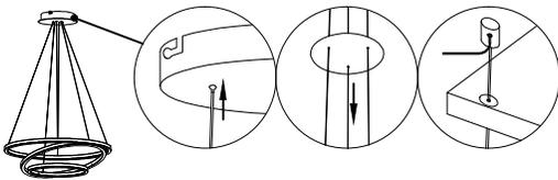
All support lines should be at the same height. Push the lock nuts up to release the lines and pull through accordingly. Release once your height is set and tighten the hex screw with the allen key on the inside of the canopy to lock the nut and keep the lines in place.
