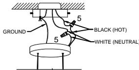
Connect the hot wire from main wire to the hot wire from power supply. Connect the neutral wire from the main wire to the neutral wire from power supply. Connect the bare copper ground wire to the green screw on the hanger.
