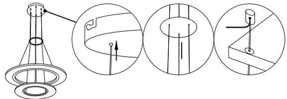
All support lines should be at the same height. Push the lock nuts up to release the lines and pull through accordingly. Release once your height is set and tighten the hex screw with the allen key on the inside of the canopy to lock the nut and keep the lines in place.
