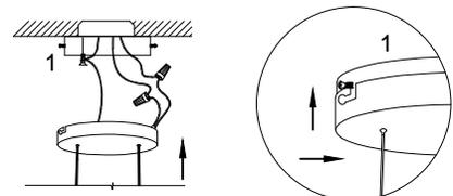
Mount the fixture ceiling canopy to the hanger by sliding the fixture cover over the hanger where the screws are sticking out on the side and twist to the right to lock into place.
