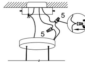
Connect the power and neutral wires using the provided wire caps (5). Connect the white wire from the fixture to the neutral wire in your ceiling junction box. Connect the black wire to the power wire in your ceiling junction box. Connect the bare copper ground wire to the green screw on the hanger.
