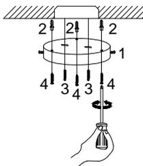
Drill the ceiling holes for the plastic anchors (2). Install the provided plastic anchors into the holes you've just drilled. Mount the hanger with the 5 screws provided. The 3/4" screws (3) are screwed into your junction box. The 1 1/8" screws (4) are screwed into your plastic anchors.
