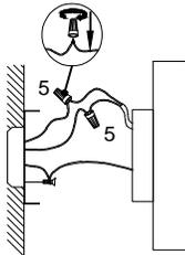
Connect the power and neutral wires using the provided wire caps. Connect the white wire from the fixture to the neutral wire in your ceiling junction box. Connect the black wire to the power wire in your ceiling junction box. Connect the bare copper ground wire to the green screw on the hanger.
