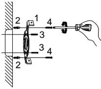
Drill the wall holes for the plastic anchors (2). Install the provided plastic anchors into the holes you've just drilled. Mount the hanger with the 4 screws provided. The 3/4" screws (3) are screwed into your junction box. The 1 1/8" screws (4) are screwed into your plastic anchors.
