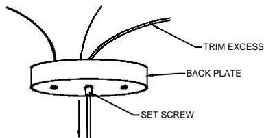
Measure the fixture to the desired height. Loosen the set screw with a small flat head screw driver. Pull through any excess power line to your desired length. Tighten the set screw and reconfirm the desired height is met. Trim excess power line leaving enough line to connect into the junction box. Strip the rubber casing to expose the wire.
