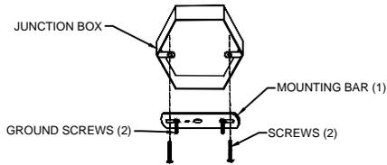
Secure the mounting bar (1) to the electric junction box with the screws (2) provided.
