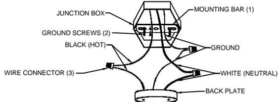
Connect the hot wire from main wire to the hot wire from power supply. Connect the neutral wire from the main wire to the neutral wire from power supply. Fix the ground wire from fitting to ground wire (grounding) from power supply.
