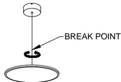
There is a break point on the light's pole. To connect the pole, thread the metal extension into the fixture collar.
