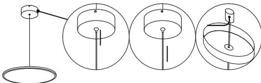
Push the lock nuts up to release the lines and pull through accordingly. Release once your height is set and tighten the hex screw with the allen key on the inside of the canopy to lock the nut and keep the lines in place.
