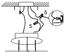
Connect the power and neutral wires using the provided wire caps. Connect the white wire from the fixture to the neutral wire in your ceiling junction box. Connect the black wire to the power wire in your ceiling junction box. Connect the bare copper ground wire to the green screw on the hanger.
