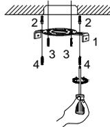
Drill the ceiling holes for the plastic anchors (2). Install the provided plastic anchors into the holes you've just drilled. Mount the hanger with the 4 screws provided. The 3/4" screws (3) are screwed into your junction box. The 1 1/8" screws (4) are screwed into your plastic anchors.
