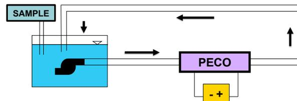
Figure 2: Schematic of one PECO unit; a 7L tank, 12V Power Supply, 2-1/2" ID x 3/4" OD Vinyl Connector Tubes, PECO device, Pump (Max Q = 5.4 L/min)
