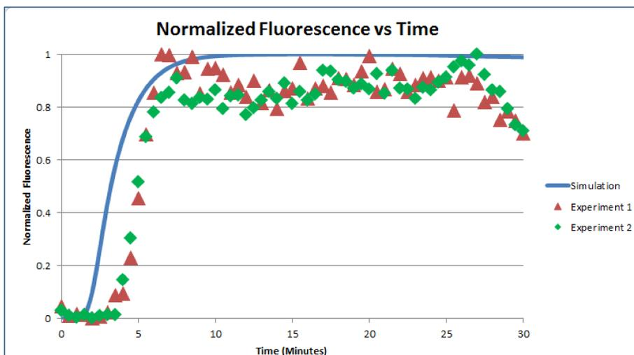
Validation plot of Simulations vs. Experiments shows a close match between the experimental results and our model
