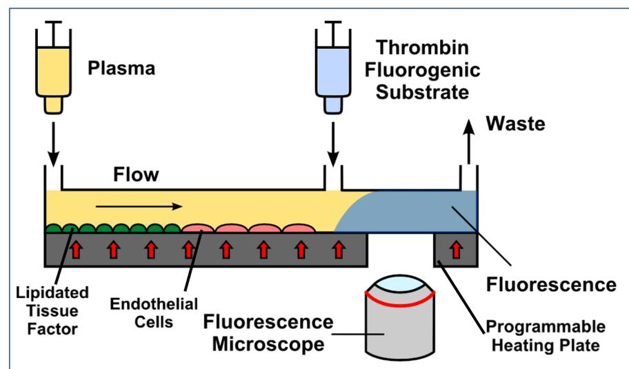
Schematic of microfluidics experiment
