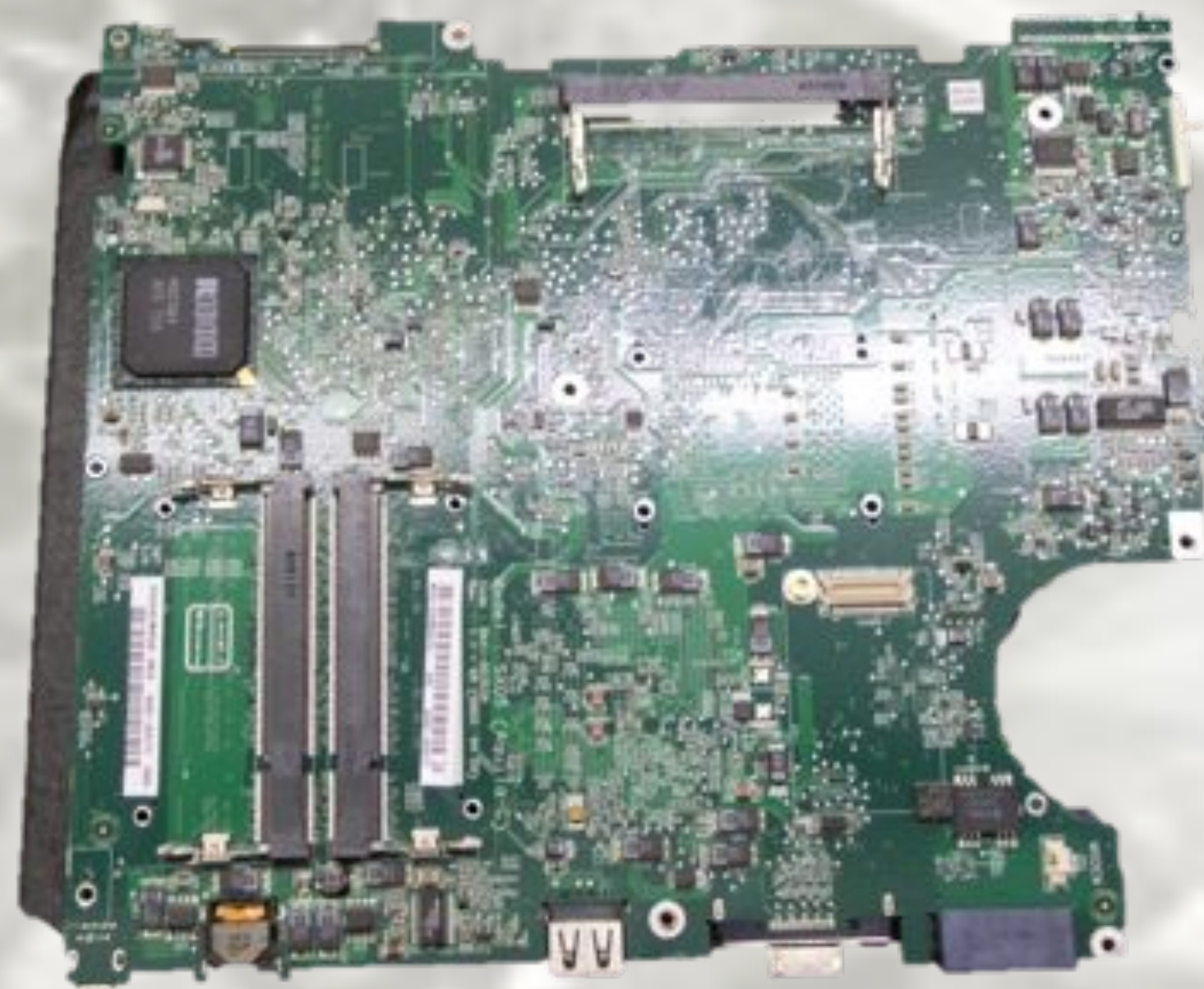
Figure 1: A printed circuit board (PCB) from a disassembled laptop. Tetrabromobisphenol A (TBBPA) is a BFR that is used in 90% of PCBs. The long term health effects of TBBPA on humans is uncertain, but known to bioaccumulate in people and the environment.
