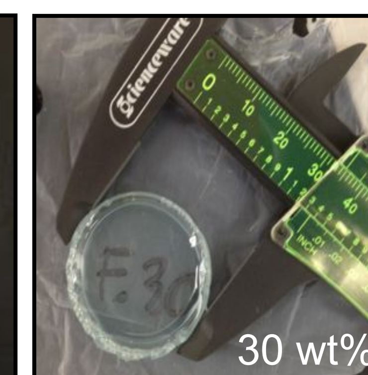
30 wt% index matched particle brush in PMMA.
