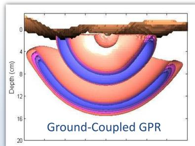
Comparison of the subsurface waveform after 7.5ns of an air-launched GPR system and a ground-launched GPR system for the same dispersive soil with a rough surface.
