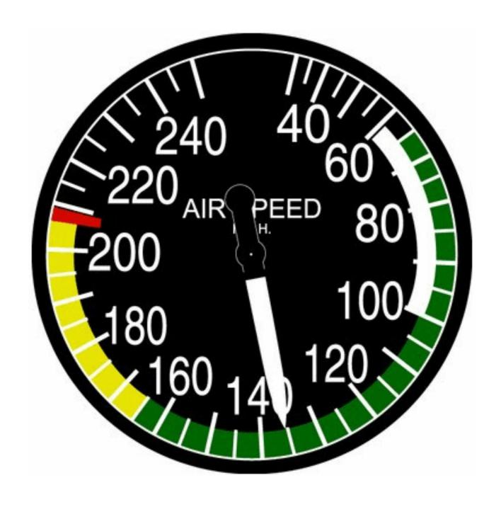
Figure 4 - Airspeed Indicator.
