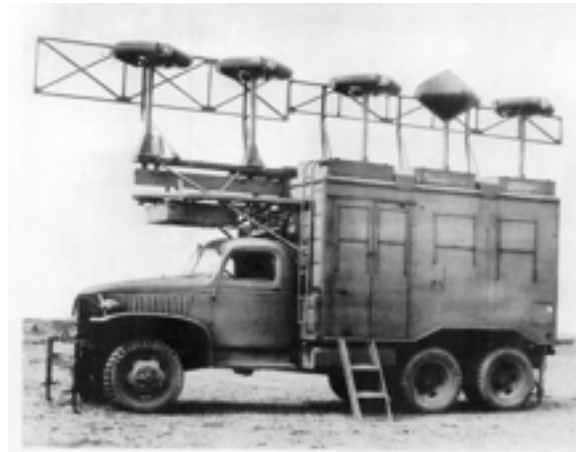
RADIO SET AN/MRN-1 TOTAL WEIGHT 16,900 LBS.
