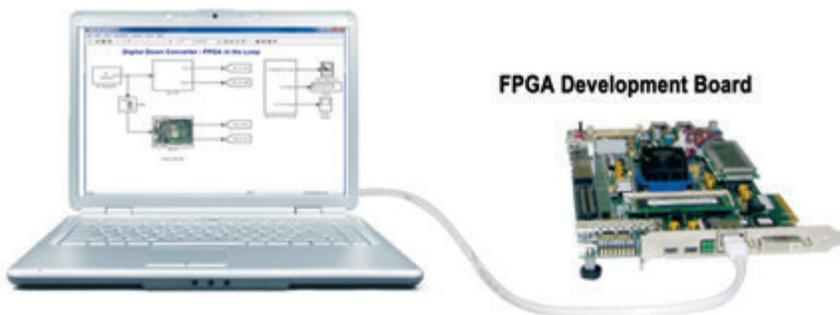
**Figure 10 - FPGA-in-the-loop simulation using Simulink and FPGA hardware.**
