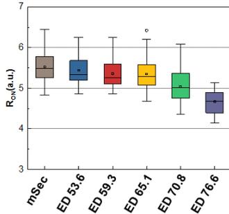
**Fig. 10.** pFET  $R_{ON}$  versus incident nSec laser energy density. Millisecond-scale (mSec) annealing serves as the reference.
