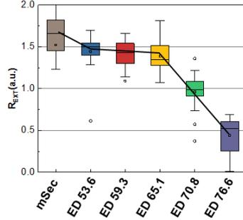
**Fig. 11.** pFET  $R_{EXT}$  versus incident nSec laser energy density. Millisecond-scale (mSec) annealing serves as the reference.
