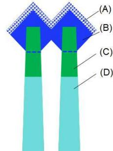
**Fig. 8.** Schematic of pFinFET highlighting materials with different melting points: (A) amorphous SiGe pocket; (B) SiGe S/D epi; (C) SiGe active fin; (D) Si subfin.
