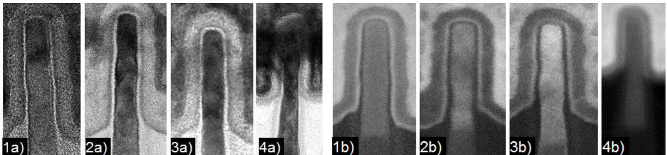
**Fig. 9.** Bright field ("a"-series) and dark field ("b"-series) STEM images of pFET fins: (1) prior to laser annealing; (2) after laser exposure at ED = 82.3 - signs of SiGe channel melting; (3) after exposure at ED = 105.3 - complete channel melting and signs of Si subfin melting; and (4) after exposure at ED = 95.7 and  $100^\circ\text{C}$  higher substrate base temperature - complete melting of fin and subfin regions and Si/SiGe mixing.
