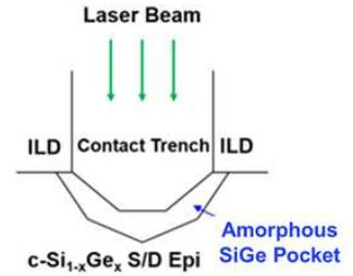
**Fig. 3.** Schematic of TLM structure for contact resistance measurement. Implanted amorphous SiGe pocket is re-grown via laser-induced LPE.
