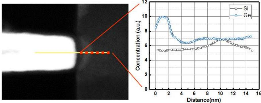
**Fig. 6.** Dark field STEM image of a formed contact using laser induced LPE at ED = 86.1.
