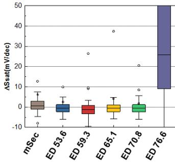
**Fig. 13** pFET change in subthreshold slope ( $\Delta SS_{at}$ ) versus incident nSec laser energy density. Millisecond-scale (mSec) annealing serves as the reference.
