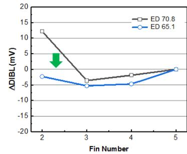
**Fig. 17.** pFET  $\Delta DIBL$  dependence on the fin number. pFETs with reduced number of fins annealed at higher temperature. Lowering incident ED by one interval eliminates DIBL degrade.
