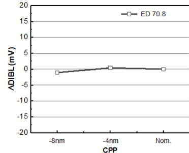
**Fig. 18** pFET  $\Delta DIBL$  dependence on the contacted gate pitch (CPP). No dependence is observed within the studied range suggesting that CPP dependence is weak.
