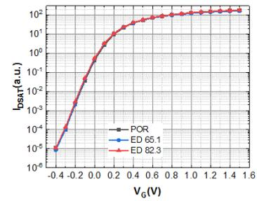
**Fig. 15** nFET  $I_{DSAT}$ - $V_G$  as the function of incident nSec laser energy density. Millisecond-scale (mSec) annealing serves as the “POR” cell.
