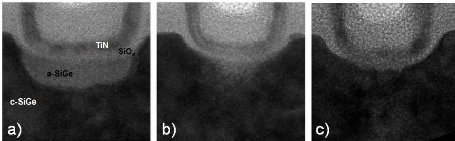
**Fig. 4.** TLM contact structures: a) after trench pocket amorphization; b) after laser exposure at an energy density (ED) of 67 - partially regrown; c) after ED = 86.1 exposure - fully regrown. ED refers to the incident energy density expressed in a.u. Laser exposure duration is  $\sim 60$  nsec. Substrate preheat did not result in a-SiGe recrystallization. TiN was used for STEM highlight without oxide removal.
