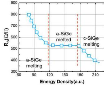
**Fig. 2.** Sheet resistance of implanted and laser annealed SiGe epi layers. Increasing laser power density results in 3 distinct regions. Laser exposure duration is  $\sim 60$  nsec.
