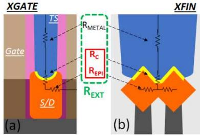
**Fig. 1.** External parasitic resistance ( $R_{EXT}$ ) in FinFETs: (a) cross gate direction (b) cross fin direction. Focus of this work is on the epi ( $R_{EPI}$ ) and contact ( $R_C$ ) resistances.
