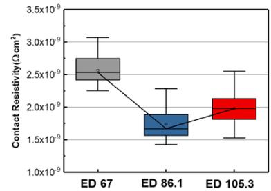
**Fig. 5.** TLM contact resistance as the function of incident energy density at laser exposure duration of  $\sim 60$  nsec. Metal stud resistance is not subtracted.
