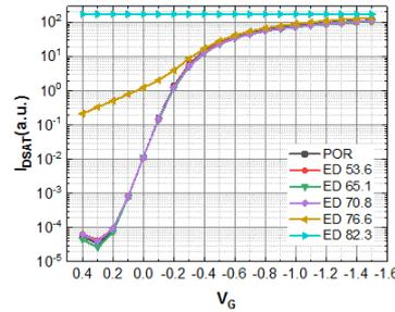
**Fig. 14** pFET  $I_{DSAT}$ - $V_G$  as the function of incident nSec laser energy density. Millisecond-scale (mSec) annealing serves as the “POR” cell.
