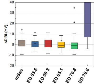
**Fig. 12.** pFET  $\Delta DIBL$  versus incident nSec laser energy density. Millisecond-scale (mSec) annealing serves as the reference.
