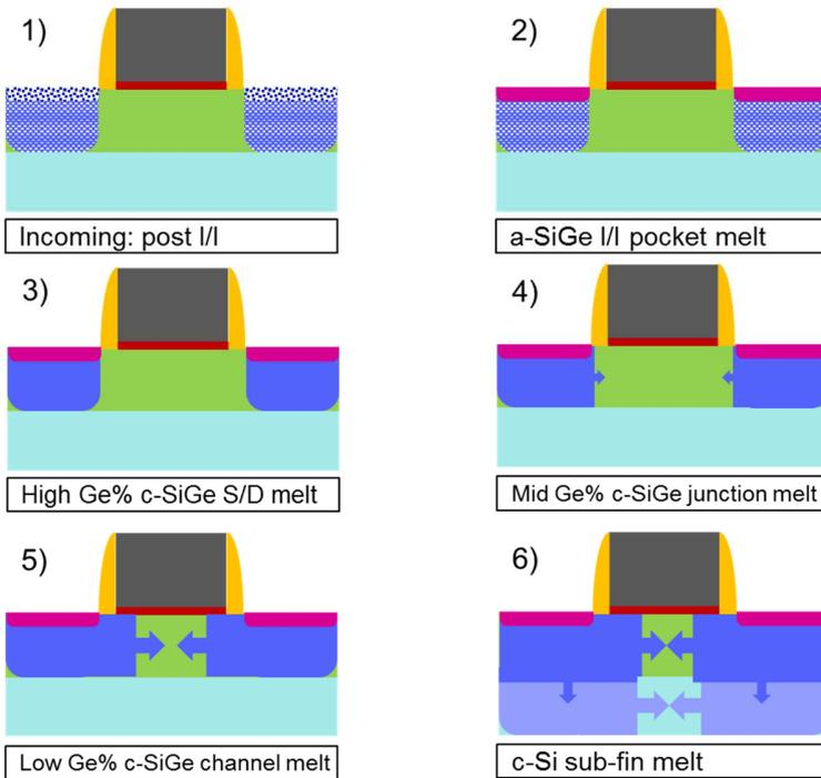
**Fig. 16.** Schematic illustrating materials melting hierarchy: (1) incoming structure; (2) amorphous SiGe pocket melt; (3) crystalline high-percent-Ge SiGe source/drain melt; (4) crystalline mid-percent-Ge SiGe junction melt; (5) crystalline low-percent-Ge SiGe channel melt; (6) Si subfin melt.
