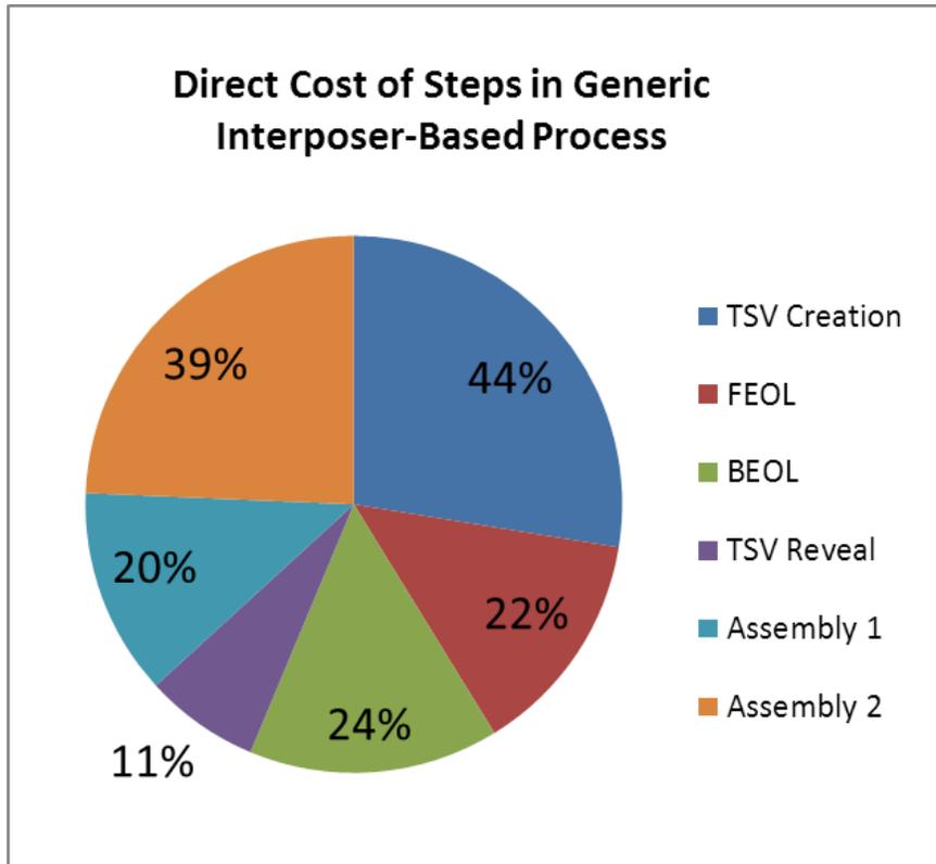
Figure 3. Direct Cost of Steps in Generic Interposer-Based Process
