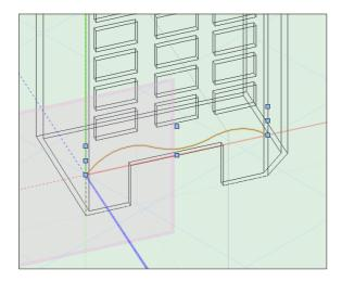
• Use the extrude command to extrude the polyline to the correct dimension.
