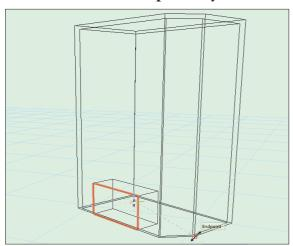
Holding down the alt or option key forces Vectorworks to use the new 3D object for solid modeling. When you move into the model, Vectorworks uses **Subtract Solid**. When you move out from the model Vectorworks uses **Add Solid**.
