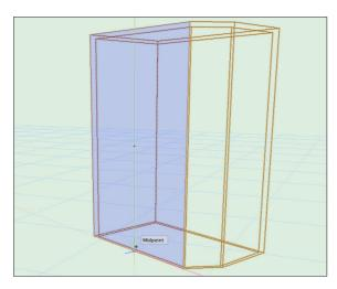
For example, you could use the Rectangle tool to draw a rectangle for the main opening on the model. Depending on the mode that you use for the Rectangle tool, you can start in the center of the model and have the center of the rectangle line with the center of your model.
