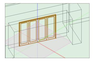
Window and door objects will not automatically create the hole in your 3D model the way they do when you place a window or door in a wall.
