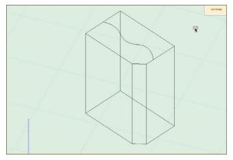
• Using the third mode for the Push/Pull tool, you can select the curve, then the model, then choose which part of the building you want to push or pull.
