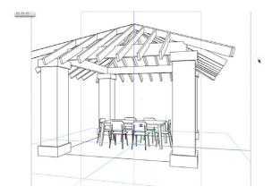
The roof framer will not make truss roofs, it will only make traditional roofs (rafters, purlins, ridge beams, and so on). If you want to make a roof with trusses, you have two options; you can create hybrid symbols for your trusses, or you can use the truss plug-in (http://www.vectordepot.com/older\_plug-ins.html) available online.
