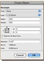
• Create a small rectangle, just 2" (50mm) high and 7.5" (190mm) wide. This will create a lip for the blockwork (CMU) to sit on.
