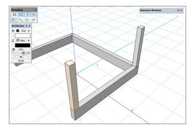
• The next part is to mirror the two columns that are already created, but they both need to be selected. While still using the **Mirror** tool, you can use the **Command** key on a Macintosh or the **alt** key on a Windows machine to select objects. Because we already have one column selected, remember to use the shift key is well so that both columns end up selected.
