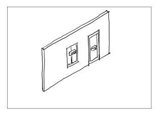
When you use 2D drawing methods you have to draw the wall and plan and you have to project the plan down to create the elevation. This is reasonably straightforward and quick. If you are used to drawing in 2D, you might use rectangles, copy, paste, guides, et cetera to draw this.
