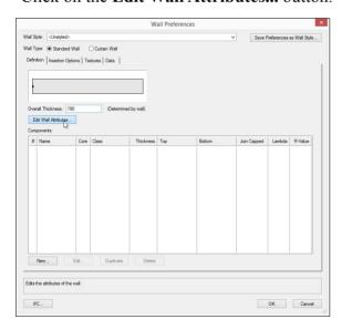
• Set all the attributes to use **Class Style**. The reason we want to use class style is so that we can easily control the line weight infill of the wall by its class and we will be able to change this on different viewports.
