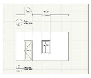
If you draw the same project in 3D, the wall is quickly drawn. The door and window tools make inserting them a breeze. Instead of creating the plan and elevation directly you would use viewports to create the same drawing as the 2D one. The 3D is just as quick to create – it just uses different tools and techniques.
