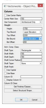
• If you are using the Vectorworks Architect levels, you can set these levels so that the bottom of the column will sit automatically on the top of the walls and the top of the column will line up with the underside of the beam above
