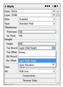
• If you are using the Vectorworks Architect Stories and Levels, go to the Object Info palette and check the Top Bound. It should be set to the level that you have created for this purpose.
