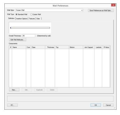
• I have also set this wall up so that it will sit directly on top of the lower wall and finish at the underside of the beams above. You could save this wall as a wall style which will allow you to use it on other projects.
