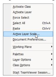
• Choose an appropriate scale for this project. I usually choose a scale which is the same as the output scale on my drawings. For example, if I want to print out my drawings at 1:50, I will set my active layer scale to 1:50. The reason I do this is that it makes things like dimensions and text easier to control because they will be created at the right size for outputting.
