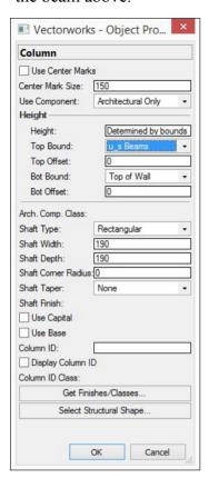
• Move your cursor on top of the wall to place the column. You might notice that I've chosen the back corner. The insertion point of the column is the centre, and moving to the intersection of the two walls allows me to snap to the centre of these walls.
