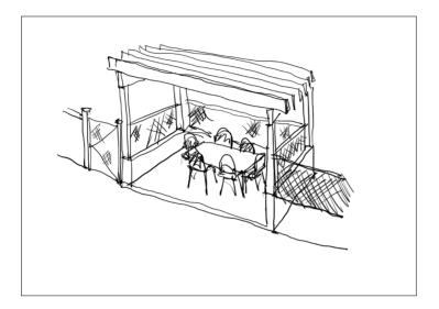
This project is so simple we could easily draw this in 2D to create a plan, roof plan, elevations, and sections. The symbol design will allow us to compare the 2D only method with the BIM concept. With the BIM concept, not only do we create plans, sections, and elevations, but we can also extract data from the model such as the volume of columns, the areas of walls, the volume of the slab, et cetera.
