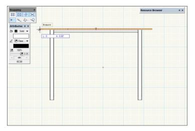
• Move down to the required position for the last rafter. In this case I have chosen to line up with the start of my rafter and the end of my beam.
