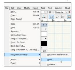
• Choose the appropriate units for your project. In this manual I am using millimeters.
