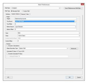
• If you are using the Vectorworks Architect Stories and Levels, set the Top Bound to be the level that you have created for this purpose. It will then connect the height of your wall to this level and if you go back to your Stories and change the level elevation, the wall will automatically change its height. This is also an easy way of controlling the height of your walls.
