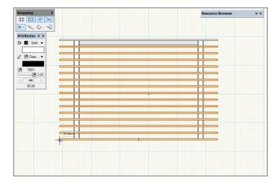
• It is a good idea to assign your walls, columns, beams, and rafters to the appropriate classes so that when you create drawings you can choose to hide some of these objects. While you're assigning these objects to classes you could also use the classes to control their textures.
