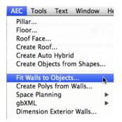
Choose to constrain tops of walls, using the geometry on the Mod-Roof layer.
