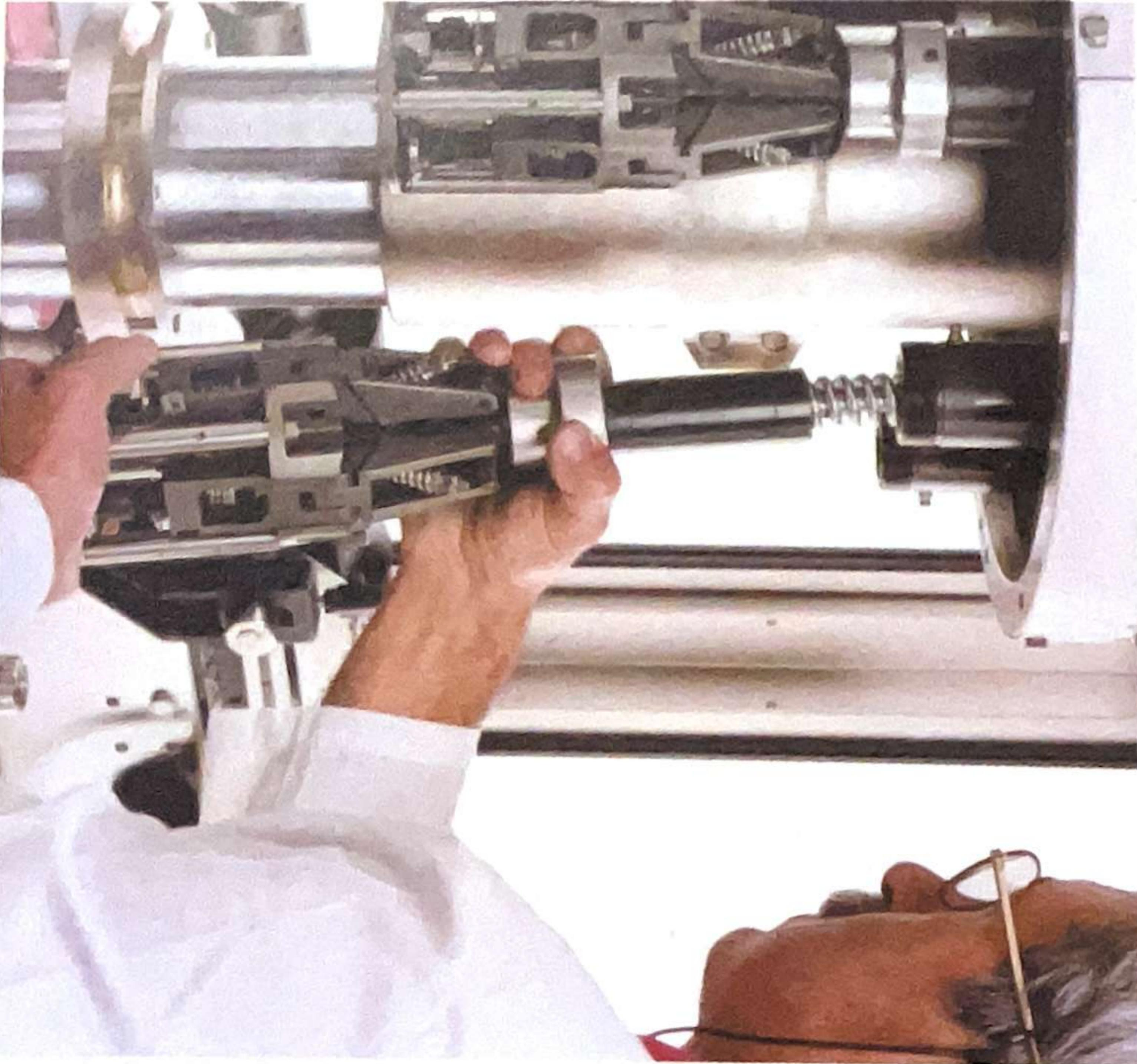
The SIGMA series is the result of years of study and research by Bertolaso in the manufacture of automatic rotary capping machines for applying aluminium caps to be threaded, press-on caps, prethreaded plastic caps and special caps.
