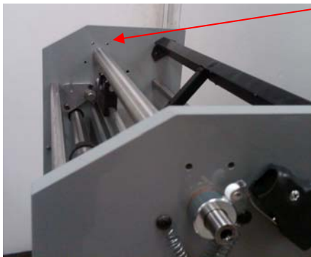
Use the button head adjustment screw to the 5 o'clock position.
