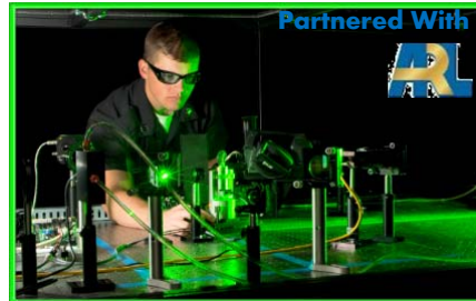
Cadet Jordan Smith aligns High Energy Laser test equipment in order to illuminate a steel target model of an 81 mm mortar round.
