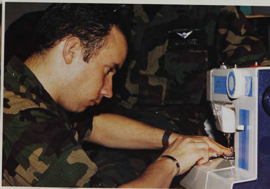
CIC Jac Coil and CIC Mike Jamoom put the finishing touches on the thermal blanket. The thermal blanket will help control the temperature of the satellite while it's in space. Photo by C. Willis.
