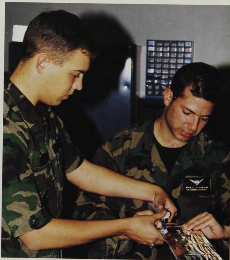
CIC Jac Coil and CIC Mike Jamoom put the finishing touches on the thermal blanket. The thermal blanket will help control the temperature of the satellite while it's in space. Photo by C. Willis.
