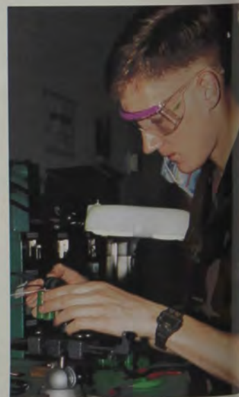
C1C Jason Clark assembles the battery packs that will be used to power the satellite. Non-rechargeable primary batteries were used in the power system. Photo by C. Willis.
