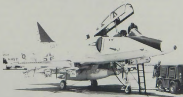
△ Recent flight tests have shown that the Marine Corp A4M armed with the Hughes-built Angle Rate Bombing System (ARBS) can significantly improve day and night bombing accuracy of Marine aircraft. ARBS uses a laser designator such as the Hughes MULE or its TV tracker to provide target acquisition.
