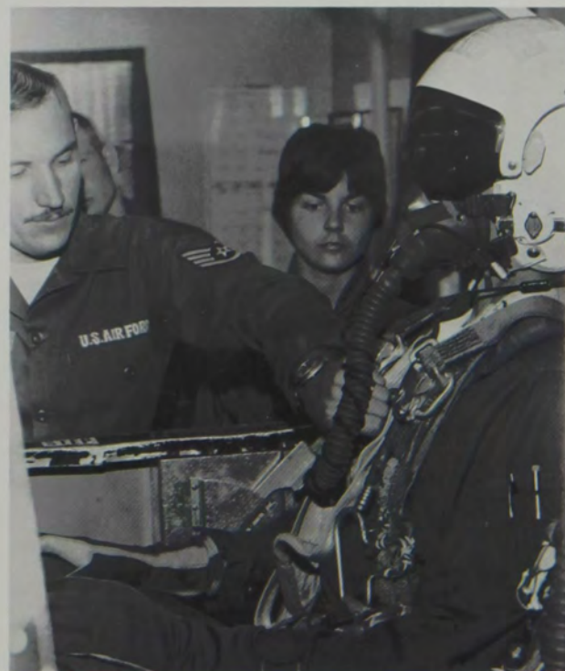
Emphasizing emergency ground egress procedures, SSgt Goodman checks radio and oxygen connection in the T-37 cockpit simulator, (RIGHT). Crew chief adjusts the oxygen mask prior to canopy closing, (ABOVE).
