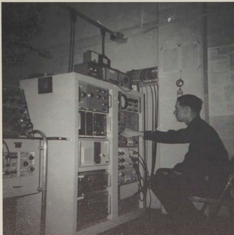
Cadet Gerald Bolme at work with the gamma ray pulse height analyzer.
