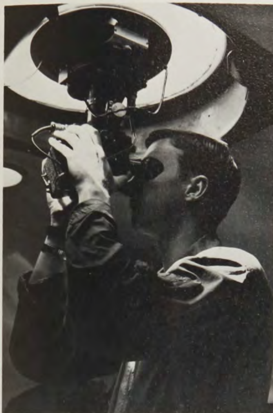
A cadet uses the sextant during a navigation flight.
