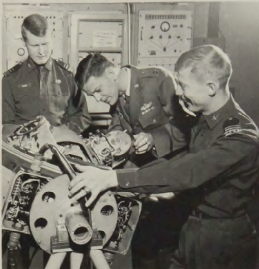
A fourteen-degree-of-freedom gyro.
