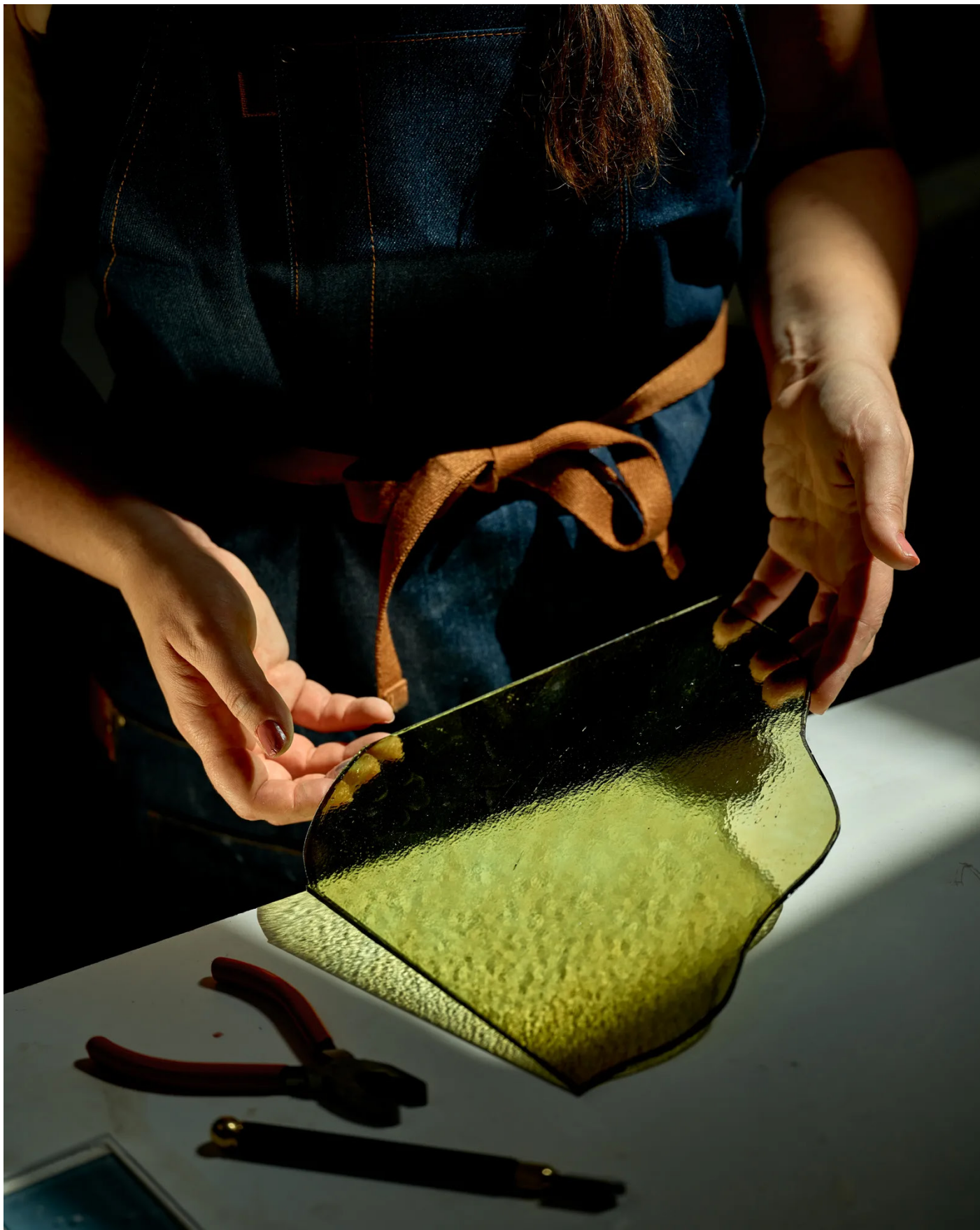
A cut sheet of olive glass that will be slump molded to create a Vera scone. Photo: Sasha Arutyunova
