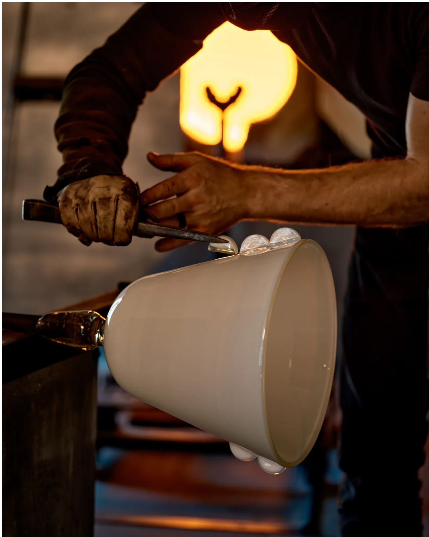
Fin embellishments are heated and fused to the Calla shade. Photo: Sasha Arutyunova
