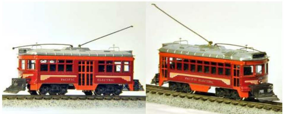
**Photo 2:** Showcase Miniatures version of a 600-series Pacific Electric "Hollywood" car on a Kato B-B power chassis; note the pole in the image on the right; it uses the old reliable NCAT design of shoe (or "trolley") to track overhead wire.
