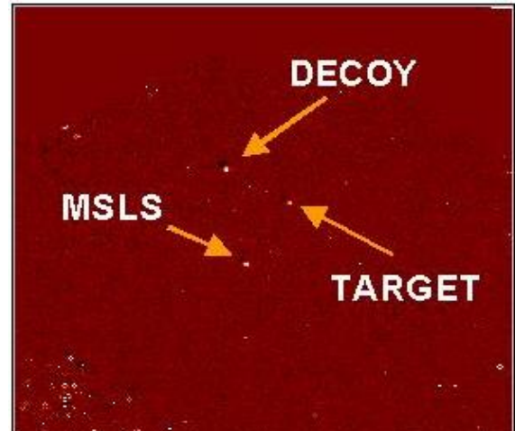
FIGURE 3. The Objects in ITF-6 as seen by the Kill Vehicle's Sensor, Roughly 90 Seconds Before Impact
