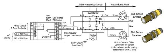
Figure 2. Hookup Using One Dual-Channel Barrier
