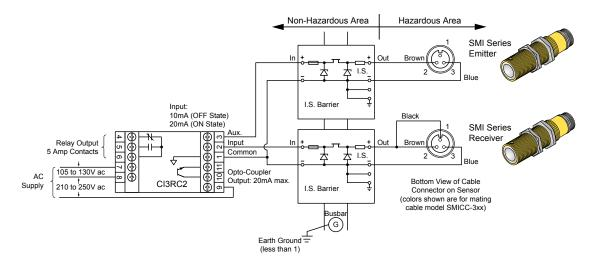
Figure 1. Hookup Using Two Single-Channel Barriers
