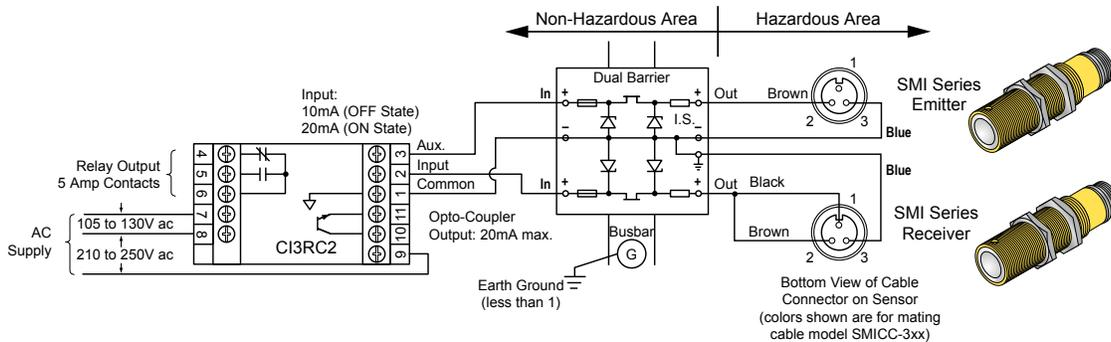
Figure 2. Hookup Using One Dual-Channel Barrier
