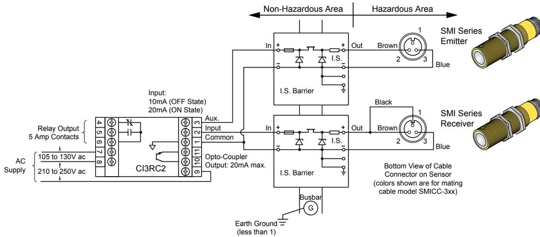
Figure 1. Hookup Using Two Single-Channel Barriers
