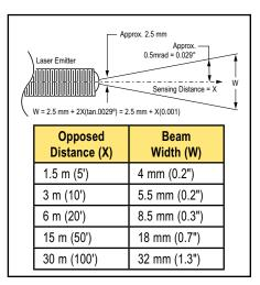
Figure 1. Laser emitter beam divergence at 25° C (beam size vs. distance)
