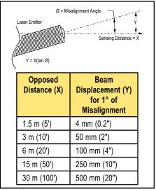
Figure 2. Beam displacement per degree of misalignment
