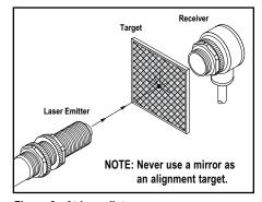
Figure 3. At long distances, use retroreflective tape to locate the beam at the receiver location.
