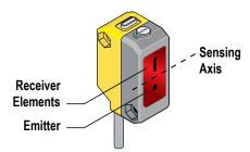
When an object approaches from the side, the most reliable sensing usually occurs when the line of approach is parallel to the sensing axis.
