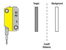
Figure 4. Set cutoff distance approximately midway between the farthest target and the closest background
