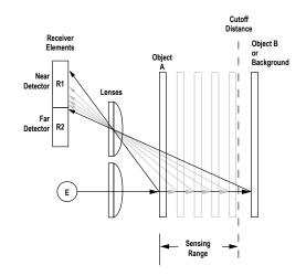
Figure 2. Adustable field sensing concept
