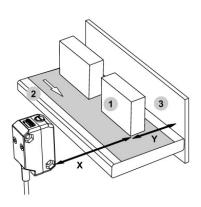
Figure 4. Background Suppression Mode Application Example
